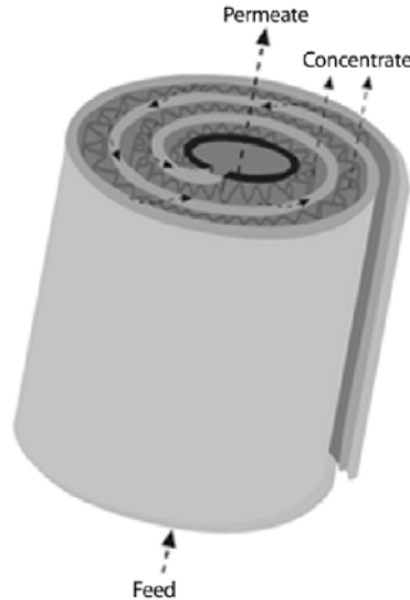
Figure 5.- Spiral wound membrane (mod. from CITME, 2006)
