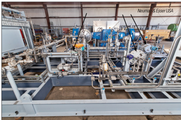
FIGURE 2. Three spiral-tube heat exchangers are shown here (arrows) within a Neuman & Esser hydrogen diaphragm-compressor package
