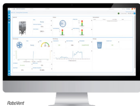
FIGURE 3. Nederman Insight is a cloud-based IIoT platform designed specifically for SmartFilter systems that provides real-time monitoring, visualization and tracking of system performance, including customized dashboards, alarms and reports
