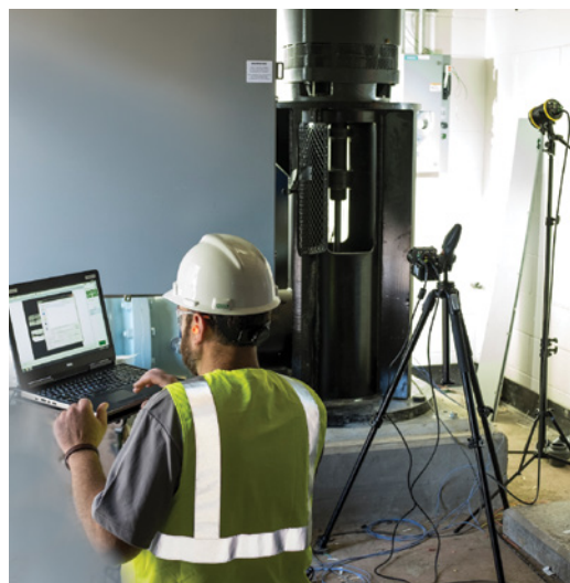
FIGURE 3. A moderate level of light and high-contrast are required for accurate displacement measurements
