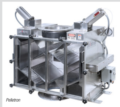
FIGURE 6. The Pelletron DeDuster uses an electromagnetic coil on the inlet to move small, micron-sized particles before the pellets are washed with air to strip those particles off the larger pellets. The process removes fines to a level well below the industry standard and enables higher-quality plastic recycling
