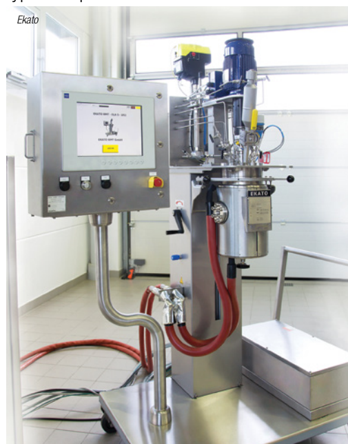
FIGURE 1. A 5-L pilot plant can be used to determine potential process limitations that are related to hydrogen-uptake rate measurement
