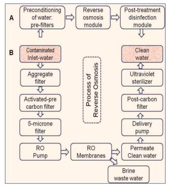
Figure 4: (A) Preconditioning/pre-filters, reverse osmosis membranes, and post-treatment disinfection system of reverse osmosis. (B) Filtration components and key steps involved in the reverse osmosis process.
