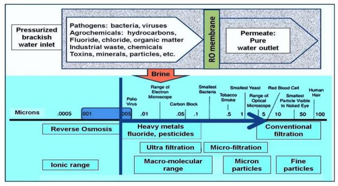
Figure 5: Detailed of various filtration methodologies and their cut-offs molecular size exclusions are illustrated. Figure indicates example of different molecules and particles that excluded with each type of filtration system.
