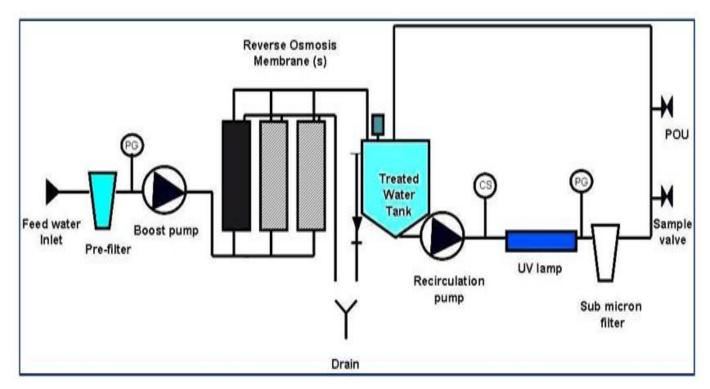
Figure 2: Basic components of reverse osmosis.
