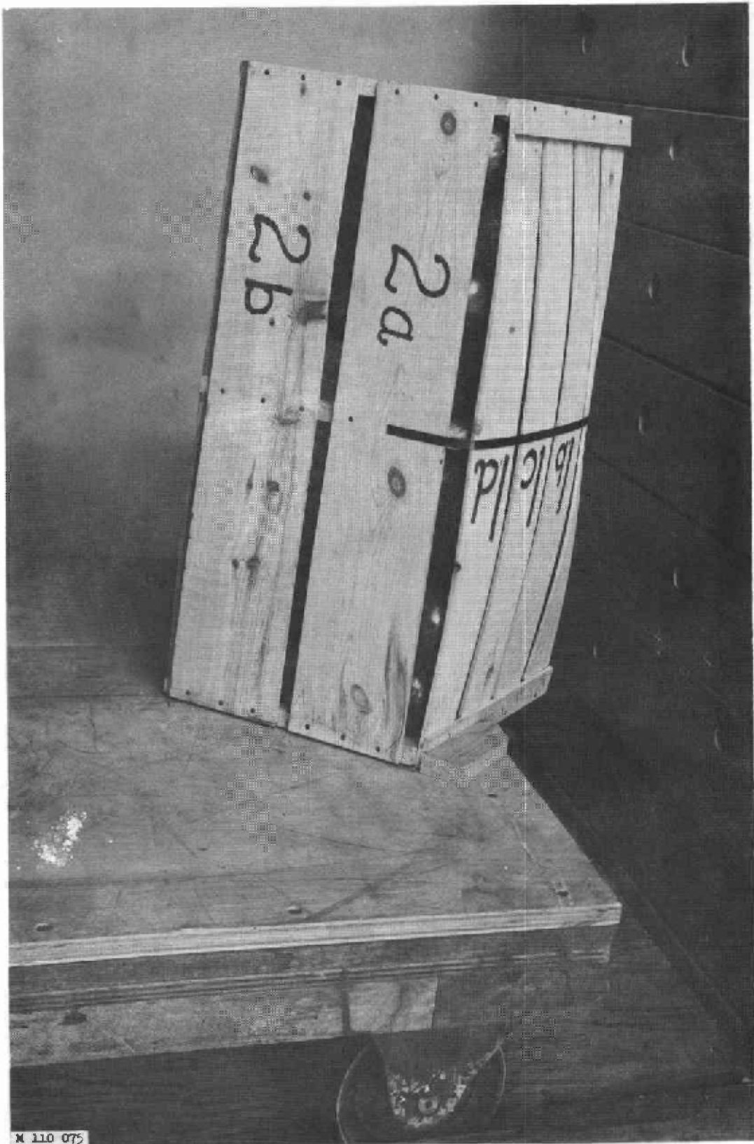
Figure 8. --Citrus box, loaded and lidded, placed on dolly in incline-impact test. Box strikes bumper at right.
