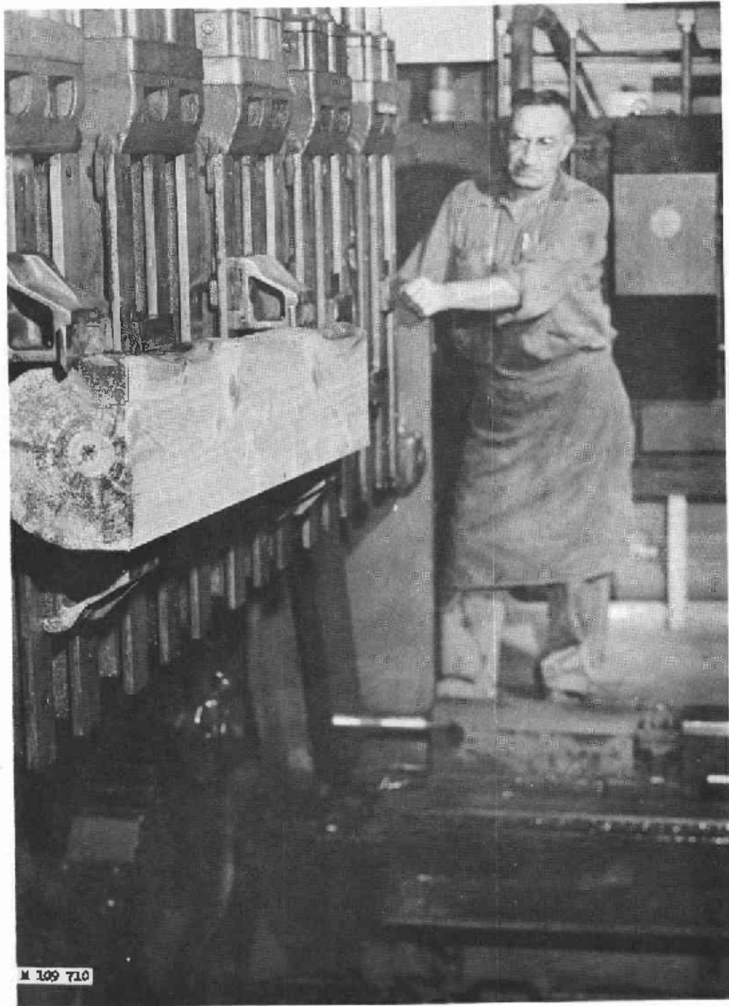
Figure 4. --Flitch mounted on slicer.
