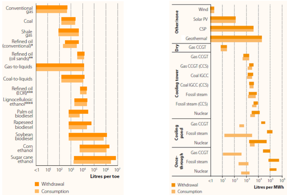
Figure 6: Water footprint of energy generation by fuel; Water use for electricity generation by cooling technology [4]
