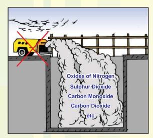
• Remove any sewage or sludge in the manhole beforehand to prevent any toxic or noxious gases that may have accumulated in it from being released and endangering the workers in the manhole in the course of their work.
