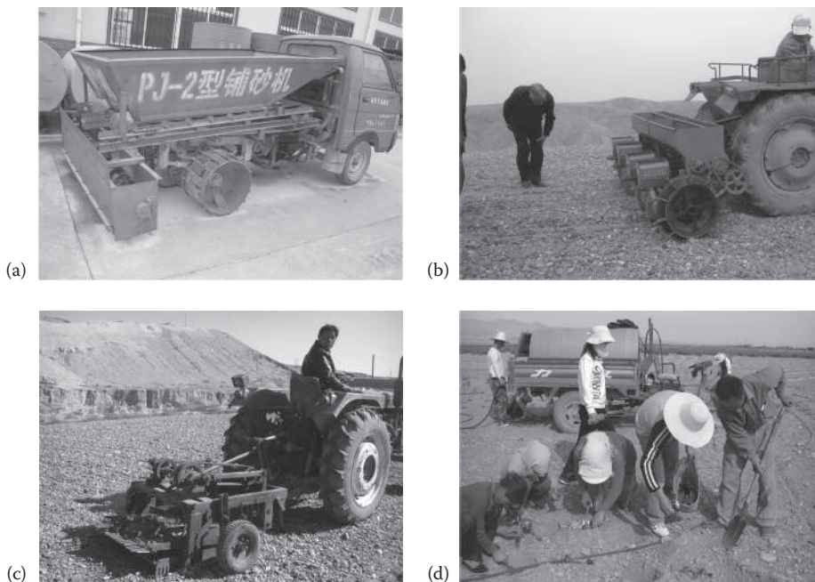
FIGURE 17.7 Machinery for shatian operations: (a) gravel/pebble-laying machine; (b) a shatian driller, which can also be used for softening the mulch layer, applying fertilizers, and sowing narrow row spacing crops (i.e., cereals); (c) gravel/pebble-sieving machine at work, and (d) farmers planting watermelon using water supplied by a water tank for supplemental irrigation.
