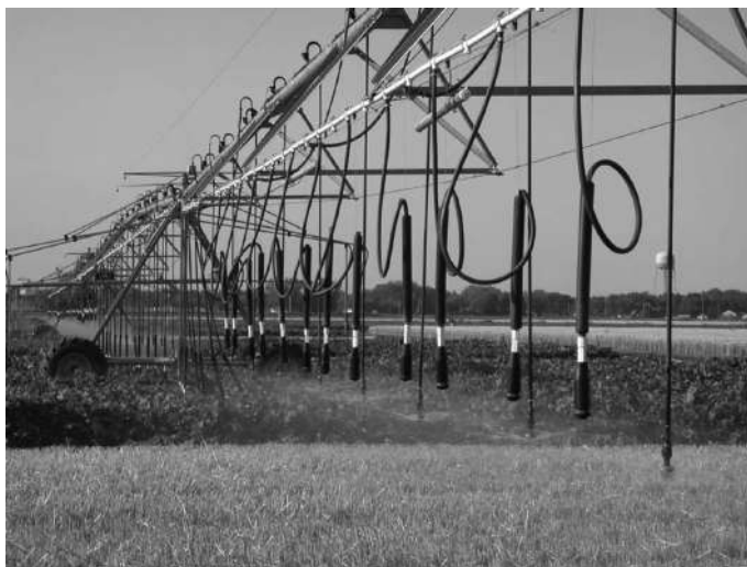
FIGURE 9.3 Dual sprinkler options (LESA and MESA) mounted on a single linear move system. (Photograph from Robert Evans, USDA-ARS, Sidney, Montana, 2010.)
