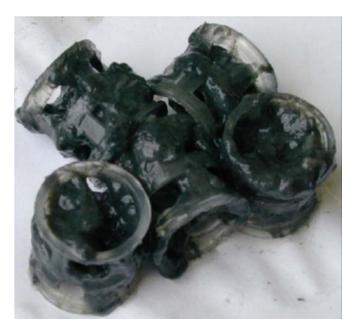
Figure 10.- Biofilm grown on SAFTEX support media. This support is Pall-rings or similar type.
