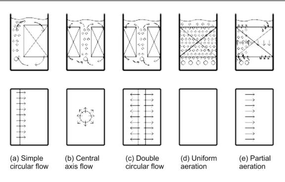
Figure 7.- Types of aeration to submerged aerated filters(Reproduced from Iwai and Kitao, 1994)
