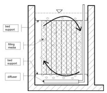
Figure 1. Scheme of a SAF process
