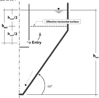
Figure 3.- Truncated cone shaped clarifier (Adapted from DWA 2000)
