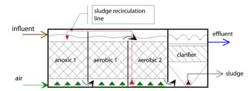
Figure 9.-Nitrification-denitrification system scheme based on 3-stage submerged aerated filters. The aeration applied on the anoxic bed is done for washing issues, as a purge for accumulated nitrogen, or even for process.
