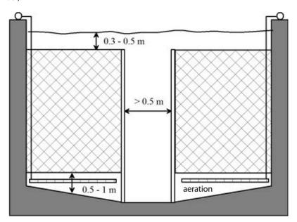
Figure 11.- Proposed configuration to design an easy access to the aeration zone for maintenance activities purpose.
