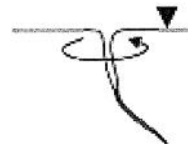
Type 4: vortex pulling in floating trash but not air
