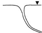
Type 6: full air core to intake
