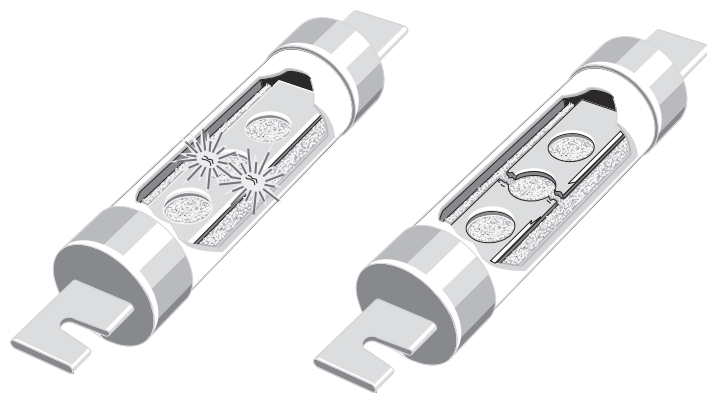
Fuse During Fault
