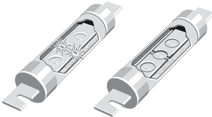
Fuse During Fault
