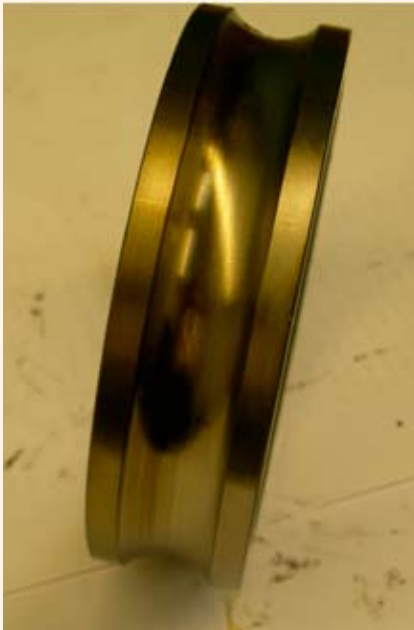
Figure 7 Photograph of Type 6217 inner ring showing running path offset from centre of raceway
