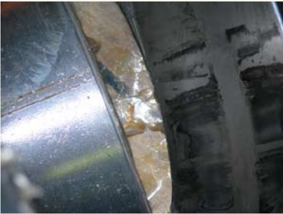
Figure 14 Type 23036 spherical roller bearing outer ring raceway showing black corrosion stains
