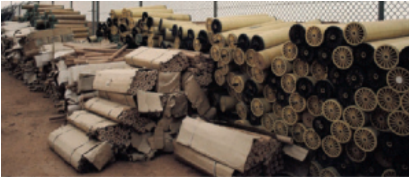
Figure 1.11 Spiral wound reverse osmosis elements and cartridge filters used for polishing RO feed water
