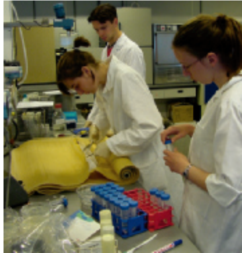
Figure 1.12 Autopsy of spiral wound membrane element for fouling diagnosis
