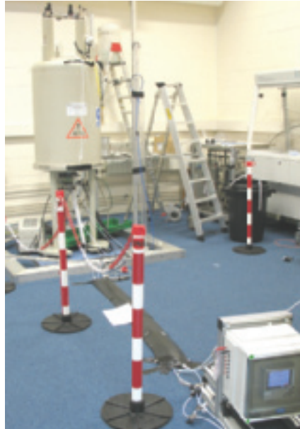
Figure 8.5 Wide-bore magnet used for the NMR study on the background, containing the S-MFS. Water containing substrate was fed to and from the S-MFS using tubing. The differential pressure transmitter (PMD70) used to monitor the pressure drop over the S-MFS is shown in the bottom right corner
