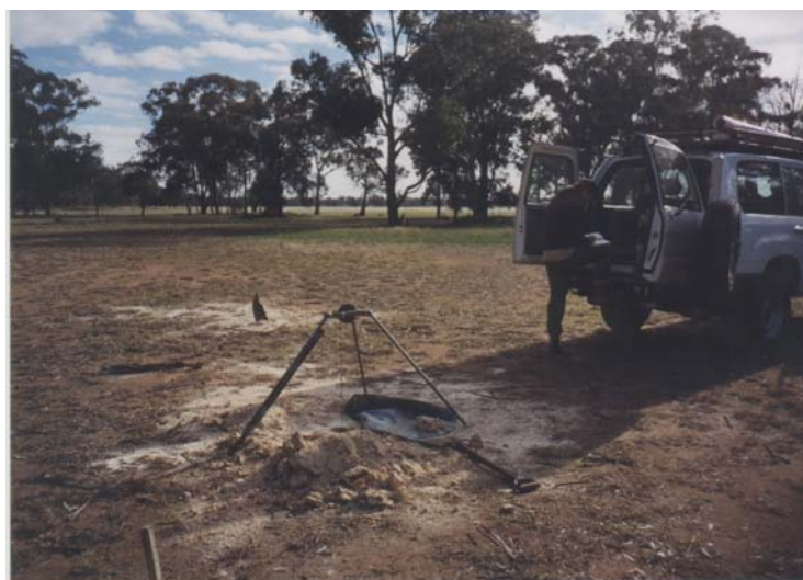
Figure 3. Regolith logging with a small, easy-to-use geophysical logging system, mounted in a 4WD vehicle.
