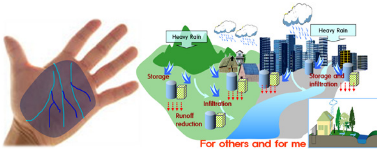
Figure 1.4 Rainwater management by area.
