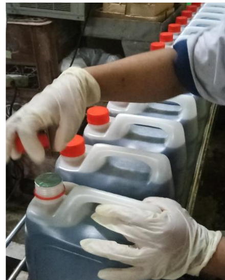
Figure 50: The checking of sealing on one of the products
