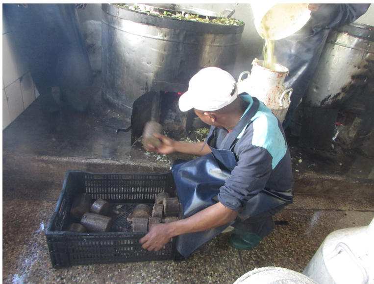
Figure 7.5 Sanivation's Superlogs being used in an industrial boiler at a flower farm in Naivasha, Kenya (image credit: Sanivation).
