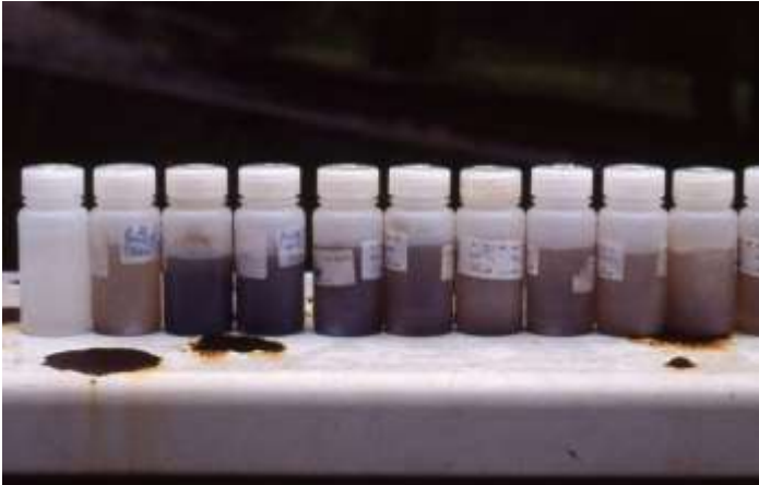
Figure 17.21 Water samples taken from a subsurface drain line when heavy rainfall followed liquid manure application. From left, water samples represent fifteen-minute sampling intervals from the onset of drain discharge. (photo by Larry Geohring).
