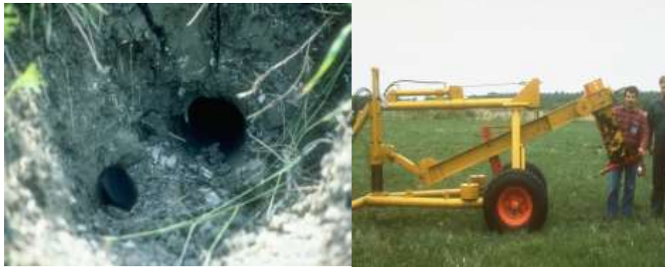
Figure 17.17 A mole drain in a clay soil (left) is created with the use of a mole plow (right).
