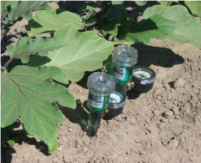
Figure 17.10. Tensiometers used for soil moisture sensing in irrigation management (photo by Irrrometer Company).
