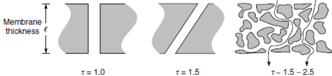
Cross-sections of porous membranes of different tortuosity
