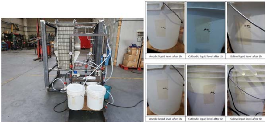
Figure 5.22 Pictures of the MDC stack and the tanks employed during the hydraulic tests. Source: Author’s own work/property.
