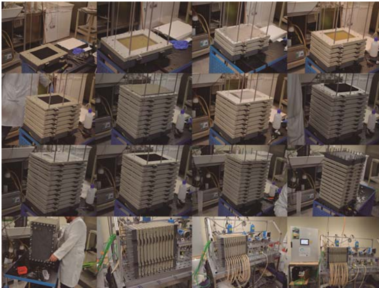
Figure 2.7 Sequence of the MDC stack assembly. Source: IMDEA Water Institute.
