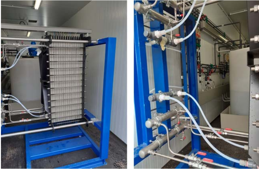
Figure 5.23 Pictures of the endplates (left) and connections of the cathodic line (right) for the second MDC stack. Source: Author's own work/property.
