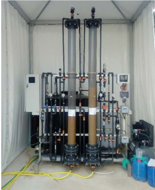
Figure 5.11 Remineralization pilot plant. Source: Author's own work/property.
