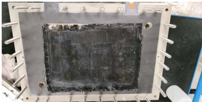
Figure 2.9 LEITAT air cathode implemented in the cathode compartment of the pre-pilot MDC system at IMDEA facilities (see details in Chapter 3). Source: IMDEA Water Institute/LEITAT.
