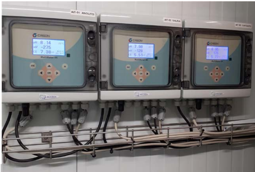
Figure 5.28 Picture of the multimeters installed in the MDC pilot plant. Source: Author's own work/property.
