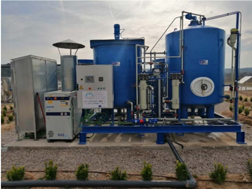
Figure 5.3 Anaerobic digestion pilot plant. Source: Author's own work/property.
