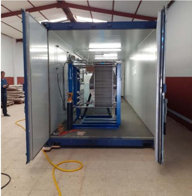
Figure 5.24 Picture of the MDC pilot plant container during integration of the peripheral elements of the installation. Source: Author's own work/property.
