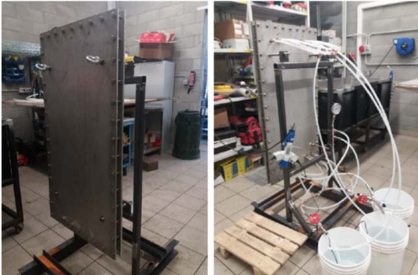
Figure 5.18 Mechanical and hydraulic testing in the single cell pilot scale MDC. Source: Author's own work/property.
