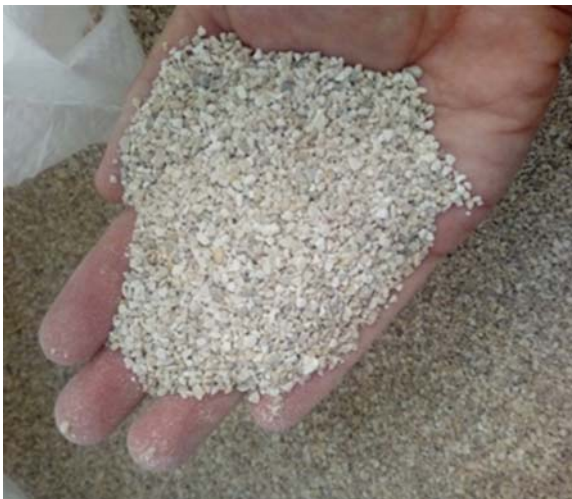
Figure 5.12 Calcite used for percolation inside the columns. Source: Author's own work/property.
