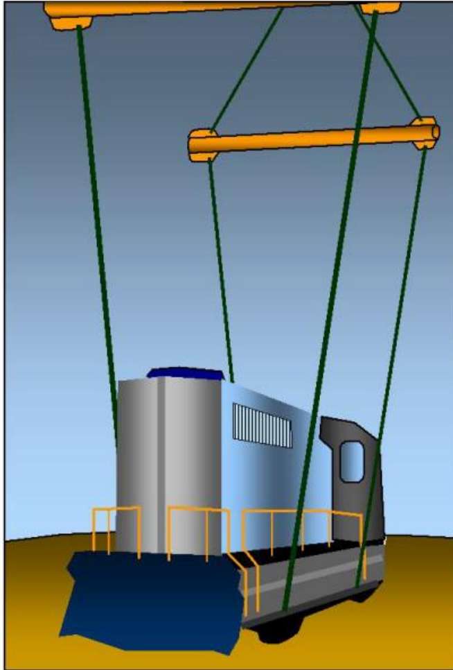
Figure 1.7: Arrangement with inward inclined secondary slings, estimated parameters
