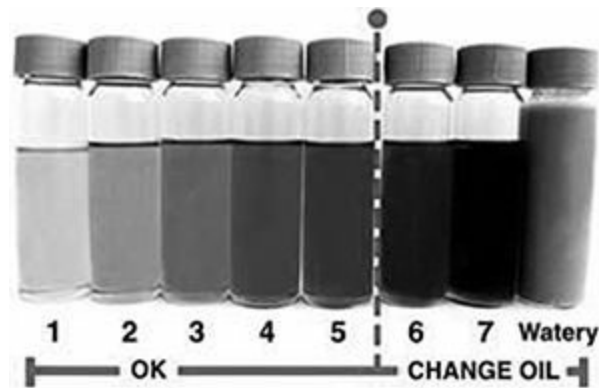
Figure 2.11—How oil appearance can change as it become contaminated. Remember look for changes from newly installed oil.
