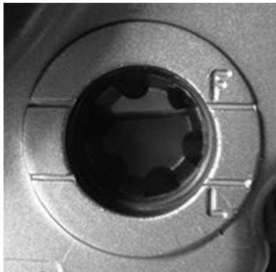
Figure 4.2—An oil level sight glass showing the full oil level.
