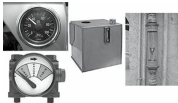
Figure 4.10—Always locate all key field instruments before starting rotating equipment. The figures shown here are of an oil pressure gauge (upper left), differential pressure gauge (lower left), level glass on a reservoir (center), and a rotameter (right)
