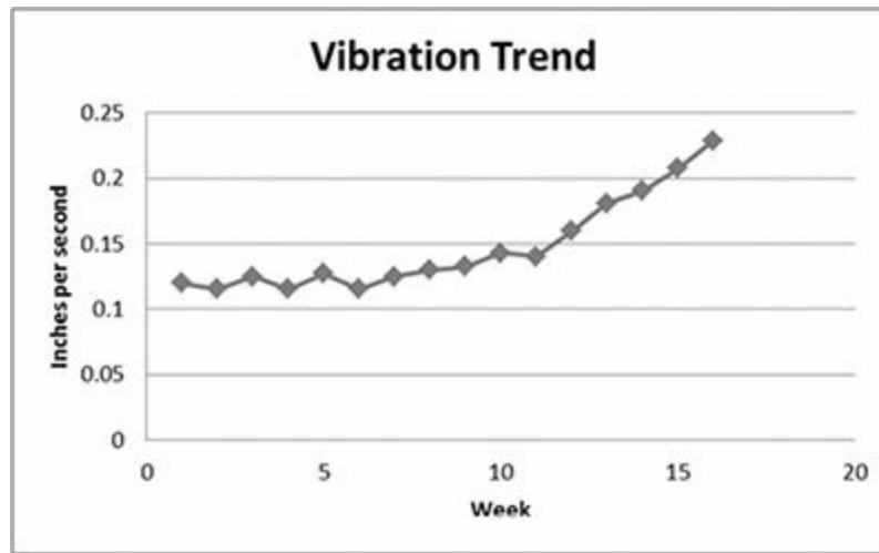
Figure 3.6—Vibration Trend Example
