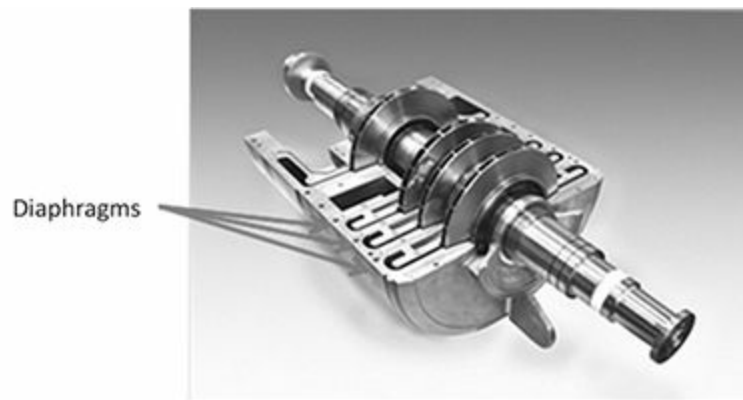
Figure 5.7—A partially disassembled multistage centrifugal compressor showing the rotor, casing, and flow diaphragms. Diaphragms guide the gas flow from one compression stage to the next.
