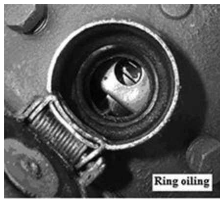
Figure 2.5—An Opened Ring Oil Inspection Port
