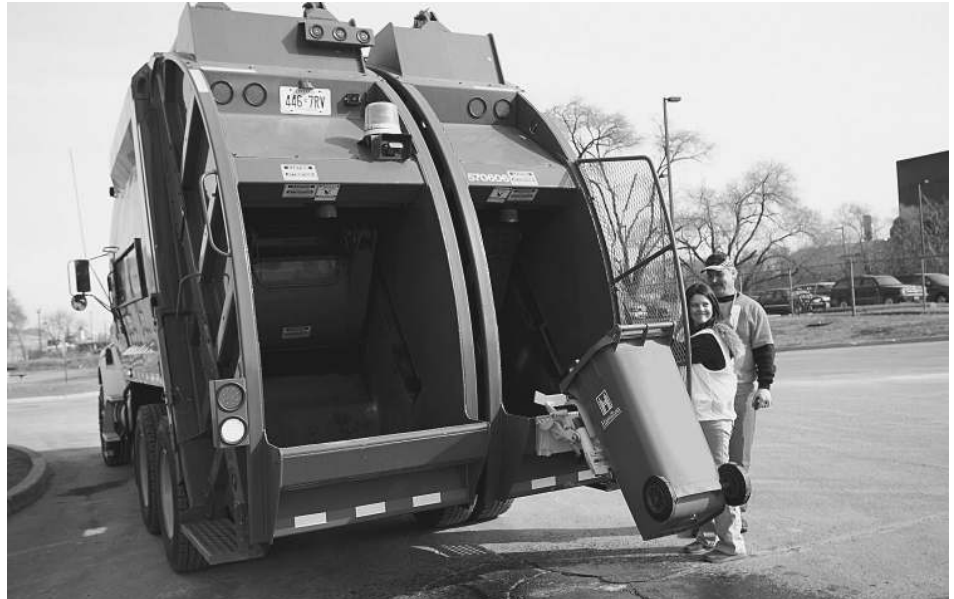
FIGURE 13-1 Dual compartment truck used in the City of Hamilton, Ontario. Conventional garbage is collected in compartment 1, while organic wastes are collected in compartment 2. (©City of Hamilton, 2007)
