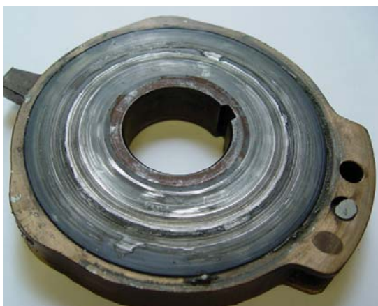
Figure 21 Oil Circulator Fused To Collar
