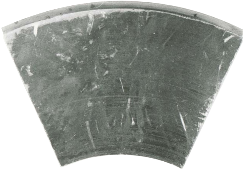
Figure 16 Tin Oxide Damage
