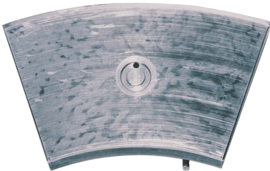
Figure 15 Thrust Shoe Surface Abrasion
