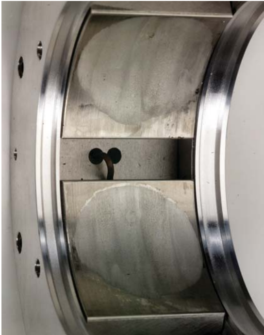
Figure 24 Stray Shaft Currents/ Electrical Pitting (Frosting)
