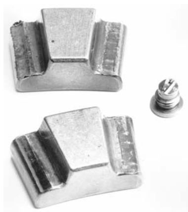
Figure 36 Leveling Plate Wear Due To Collar Wobble
