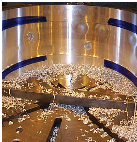
Figure 23 Large Hydrogen Blisters
