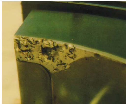
Figure 29 Eroded Babbitt From Spragging
