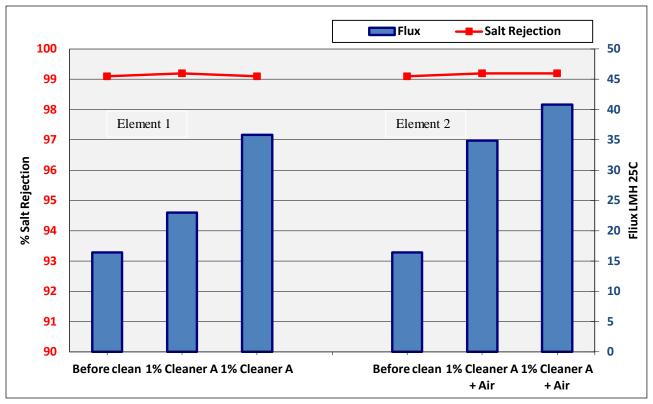
Figure 9: Graph showing effectiveness of cleaning with air
