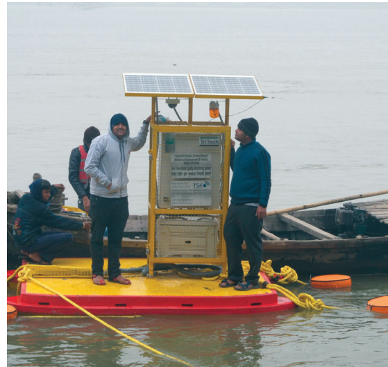
Figure 6.1: Floating monitoring station.
