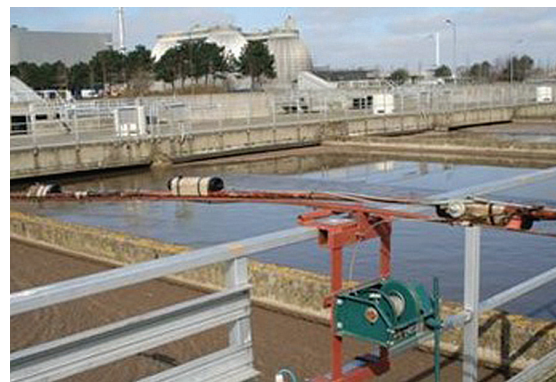
Figure 6.32: Field setup for measuring oxygen concentration profiles.
