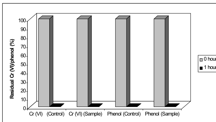
Figure 3.13: The percentage of Cr (VI) and phenol removed by the immobilized A. haemolyticus using the real mixed waste of Cr (VI) and phenol.
