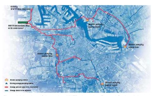
**Figure 1.1** Locations of the previous WWTPs Amsterdam East and South and the new WWTP Amsterdam West, with connecting pressure mains and booster pumping stations.
