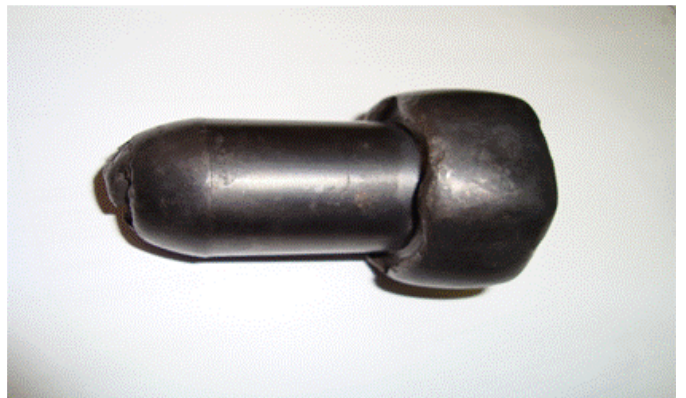
Photographs 19 to 22: Failed Non-OEM supplied BWCP components
