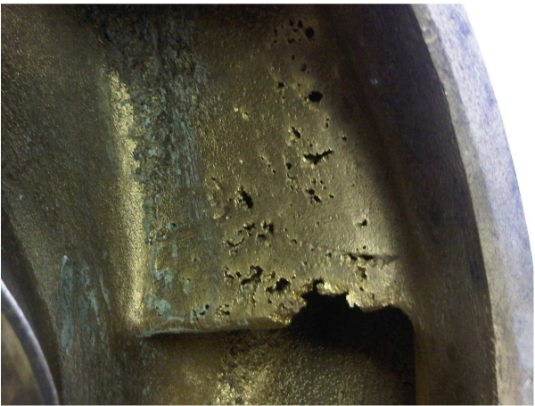
Photographs 5 and 6: Grootvlei high lift pump suction impeller - pressure side cavitation damage
