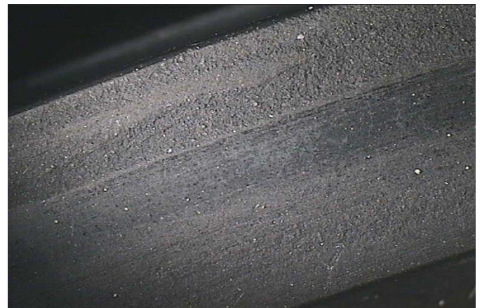
Photograph 11: Worn Carbon-Graphite seal face – "Pure" Carbon-Graphite
