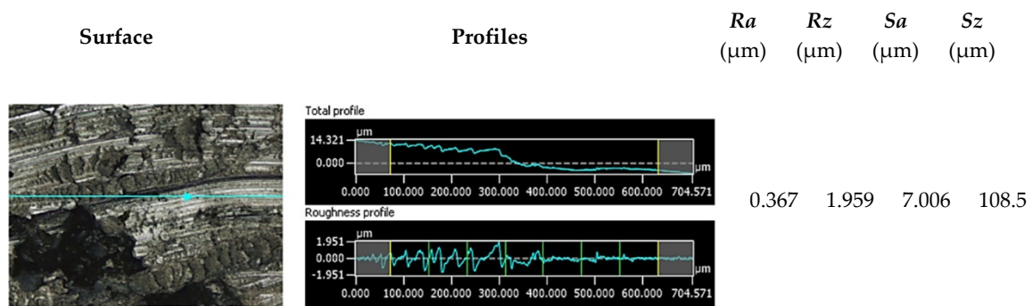
Figure 3. Example of measurement of 2 and 3D parameters of surface roughness with the Keyence microscope.
