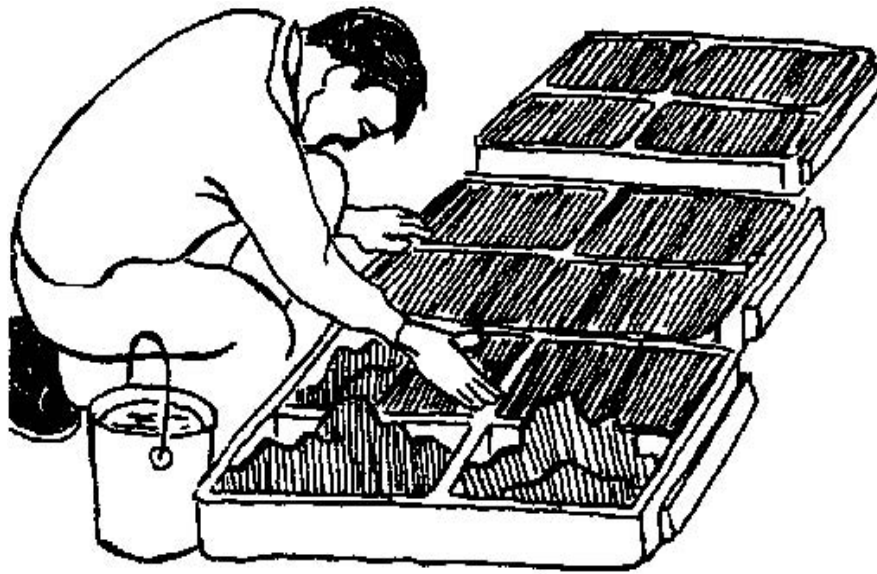
Figure 40. Kneading and leveling the blocks
