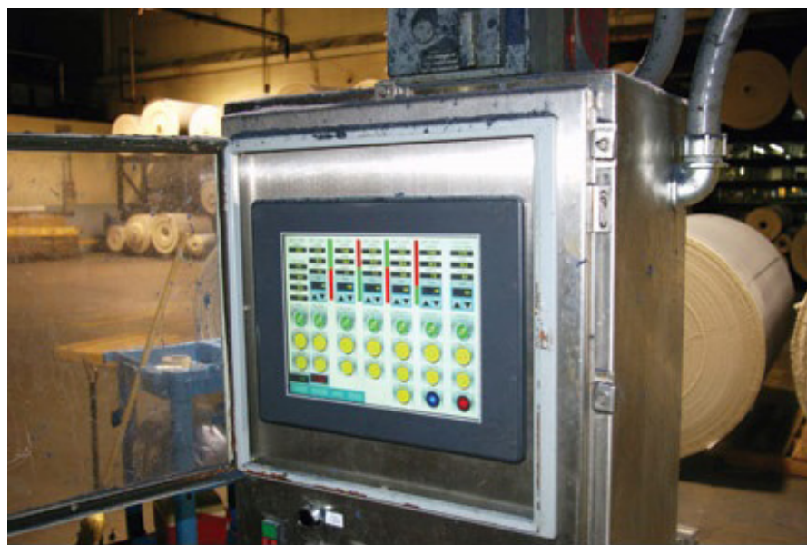
Figure 4: The 15" C-more touch screen operator interface brings all the controls of the finish line to a common point on the machine and includes set-up screens, maintenance screens, operations screens as well as diagnostics.
