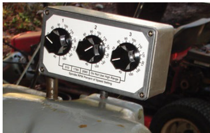
Figure 3: Three Potentiometers wired to a shielded cable
