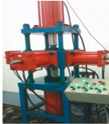
Figure 1. Self-developed true triaxial test machine.
