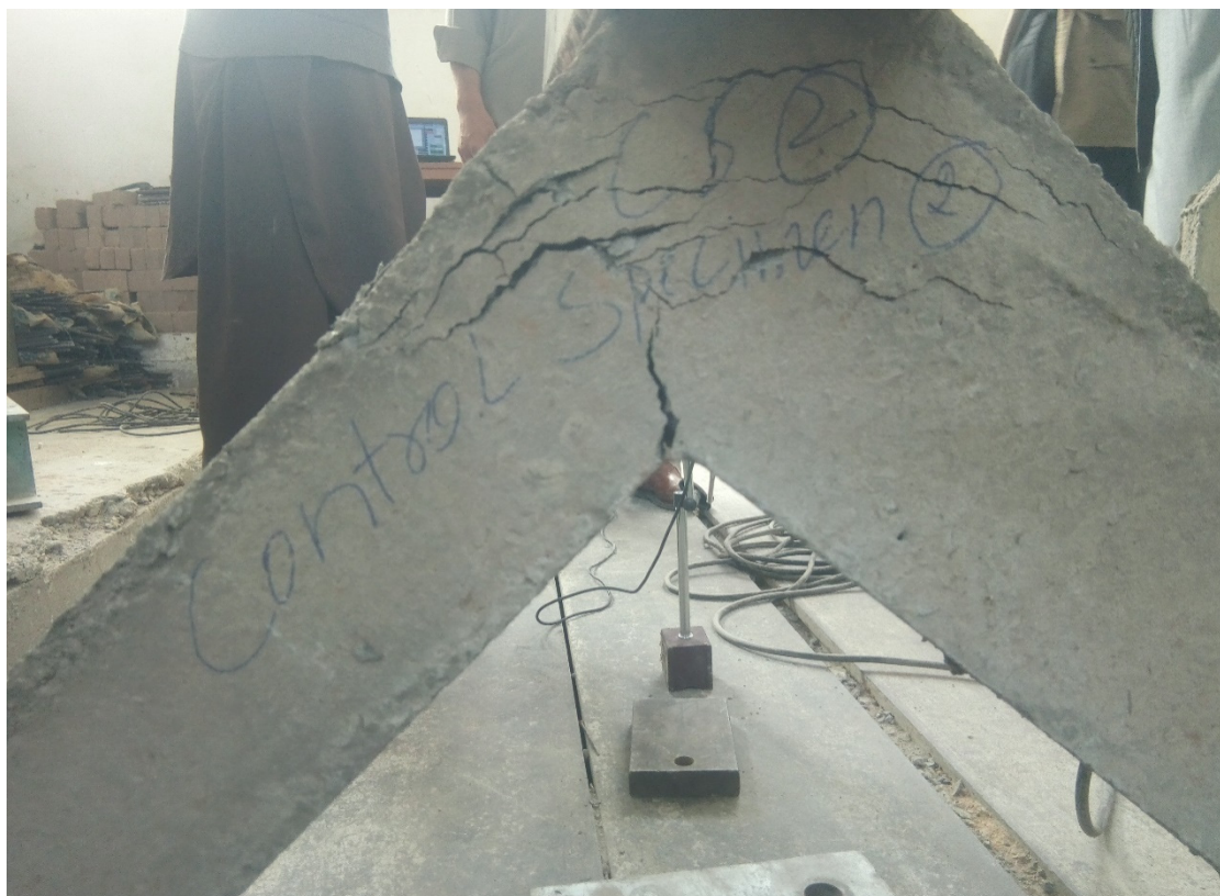
Figure 8. Failure of the conventional concrete specimen (CC_S2) after application of load.
