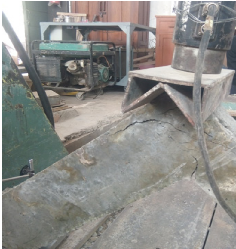
Figure 9. Failure of RPC specimen (RPC_S1) after application of load.
