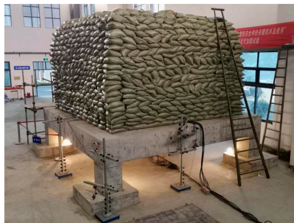
Figure 8. Pile loading of the slab.
