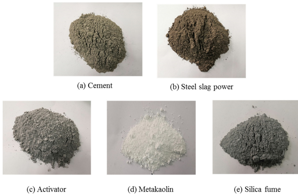
Figure 2. Samples of cementitious material components in this study (a) cement; (b) steel slag powder; (c) activator; (d) metakaolin and (e) silica fume.
