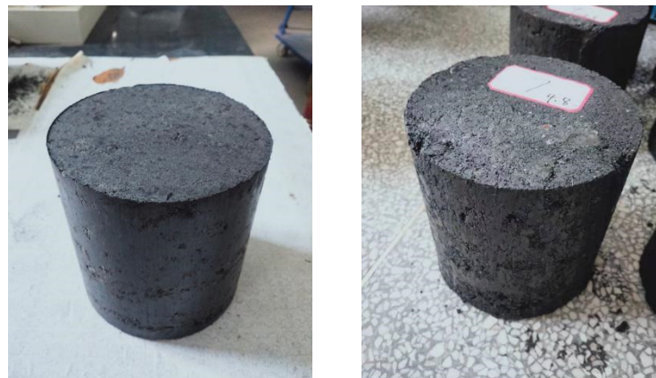
(a) Before freezing and thawing
