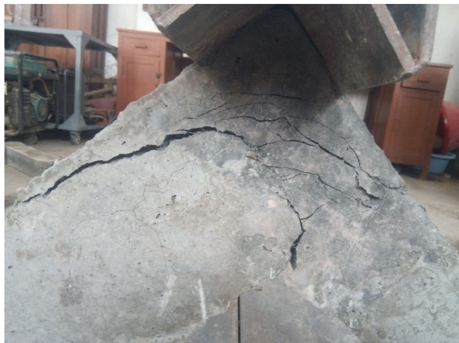
Figure 10. Failure of RPC specimen (RPC_S2) after application of load.
