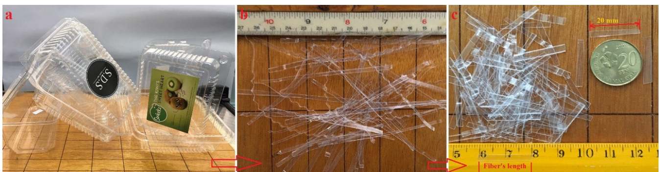
Figure 1. (a) Post-consumer waste plastic food trays, (b) fabricated fibers and (c) WPFT fibers used in this study.
