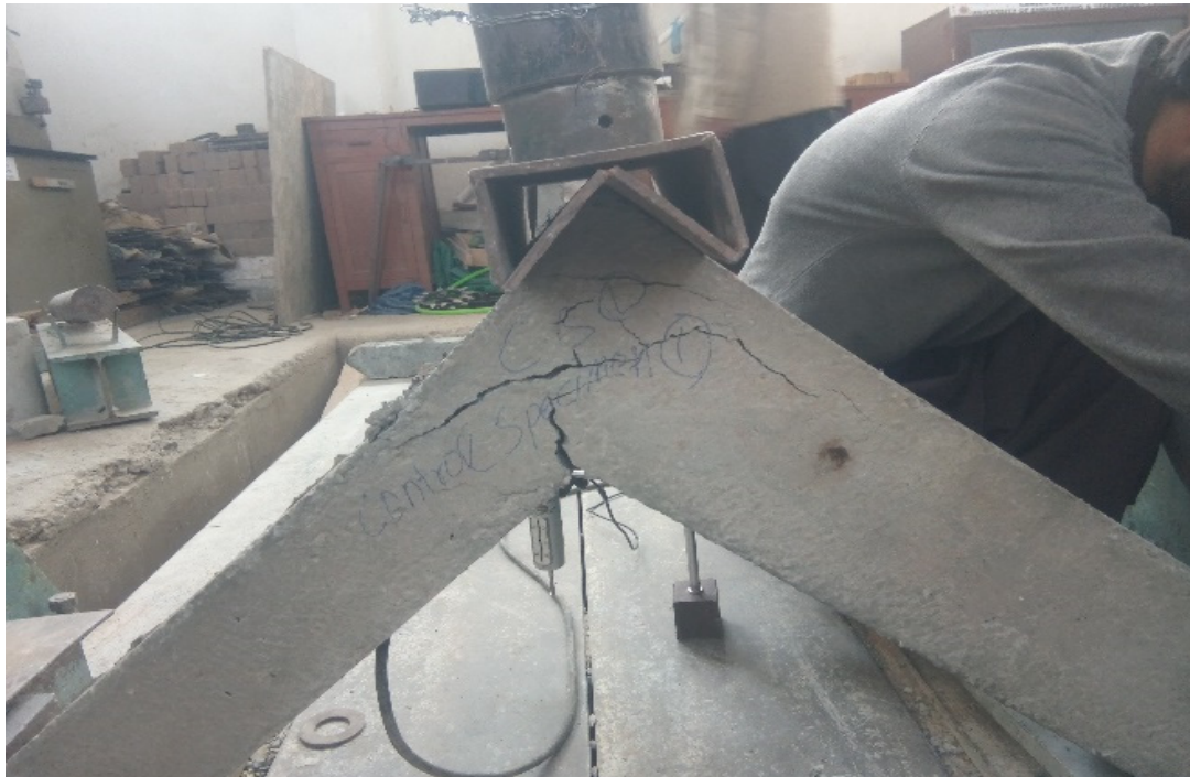
Figure 7. Failure of the conventional concrete specimen (CC_S1) after application of load.
