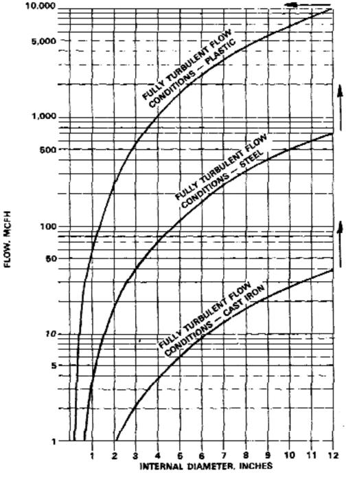
BASED UPON: IGT DISTRIBUTION EQUATION AND FULLY TURBULENT EQUATION, K=0.01 in. FOR CAST IRON, K=0.0007 FOR STEEL, K=0.00006 FOR PLASTIC, G=0.60, G=0.0105 CENTIPOISE.
