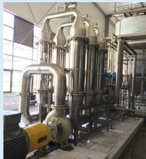
"Ceramic membrane system for beer processing, photograph courtesy GEA Processing Engineering, Inc."
