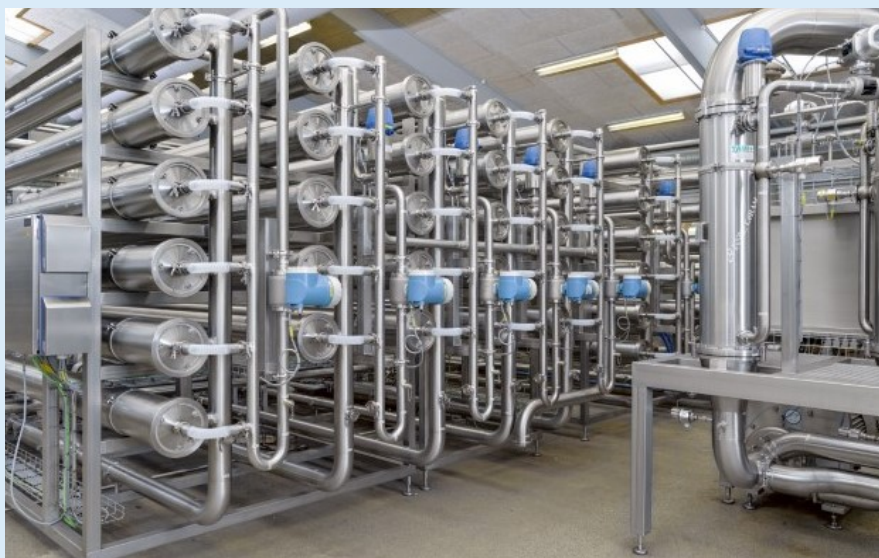
"Ceramic Microfiltration and Reverse Osmosis system for skim milk processing, photograph courtesy GEA Processing Engineering, Inc."
