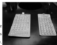
Colilert media® and sample bottle (top) and results after incubation in QuantiTrays®.
