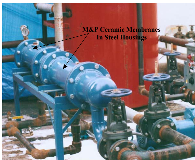
Figure 9. Used oil deashing unit featuring M&P ceramic membranes.
