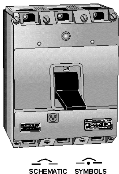
Figure 2-2.—Typical circuit breaker and schematic symbols.
