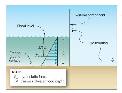
Figure 8-7. Lateral flood force on a vertical component
