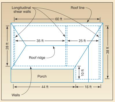
Illustration A. Building elevation and plan view of roof showing longitudinal shearwalls; dimensions are wall-to-wall and do not include the 2-ft roof overhang
