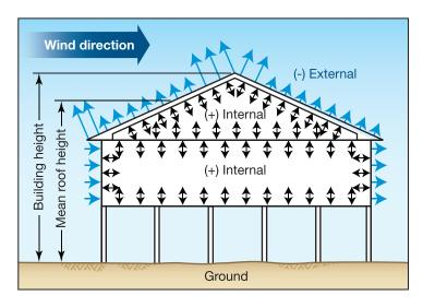
Figure 8-18. Distribution of roof, wall, and internal pressures on one-story, pile-supported building
