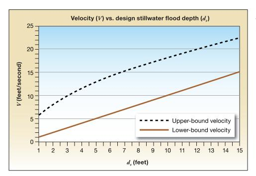
Figure 8-6. Velocity versus design stillwater flood depth
