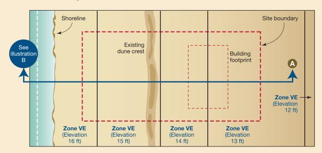
Illustration A. Plan view of site and building location with flood hazard zones
