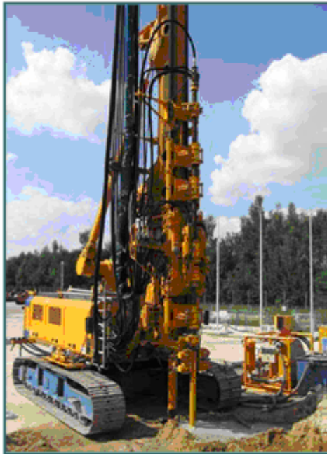
DRILLIN MACHINE BG24 USING SLURRY BENTONITE
