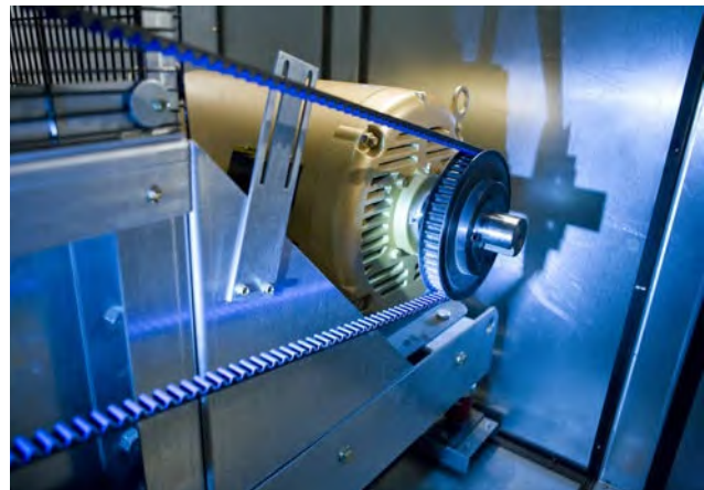
Figure 8-3. Notched and Synchronous Belts. A notched belt, left, runs cooler and has a higher efficiency than a standard V-belt. A synchronous belt, right, can maintain higher efficiency over a wide load range and requires minimal maintenance. Photos from Gates Rubber Company
