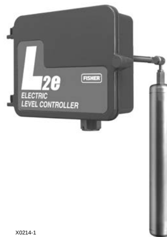
Figure 2-16. In the upstream oil and gas industry displacer type liquid level controllers along with on/off dump valves are used for controlling liquid level in oil and gas production separators. The controllers use a displacer sensor to detect liquid level or the interface of two liquids of different specific gravities. The output signal from the controller is either electric or pneumatic and sent to an on/off dump valve to open or close it. The L2e shown is the electric output version of this controller.
