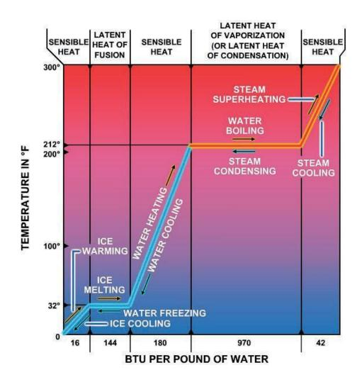
Figure 2-9 — Relationship between sensible heat and latent heat.
