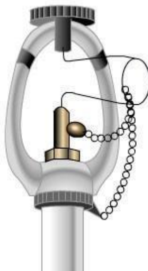
Figure 4-10 – Sprinkler pre-prime plugs.
