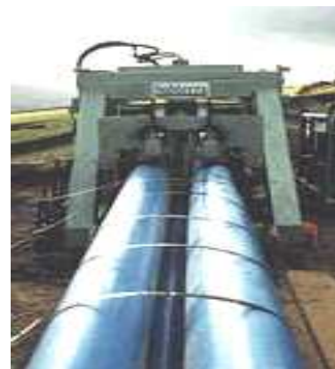
Figure 3-15. Subline Forming into “C” Shape
