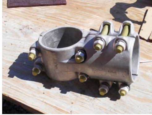
Fig. 13. Bolted Aluminum T-Conector 4"IPS Main to 4"IPS Tap
