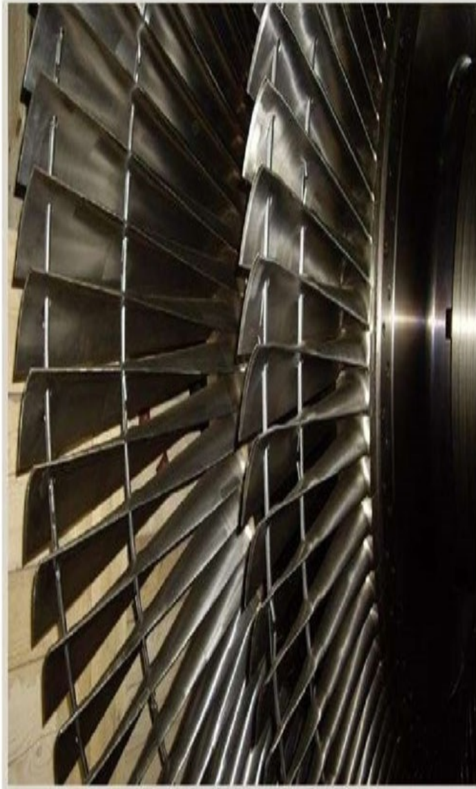
Rotor Blades showing impulse arrangement
