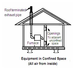
2) **Air from Outside:** If air from outside is brought in for combustion and ventilation, the confined space shall be provided with two permanent openings. One opening shall be within 12 inches of the top of the enclosure and one within 12 inches of the
