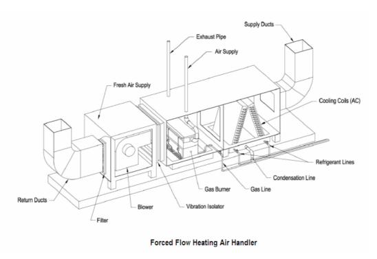
The figure above shows an air handler equipped with gas fired furnace. Another form of forced air system is the piped system using a heating coil. Instead of a gas burner, hot water is circulated from boiler to the heating coils which heat the air.
