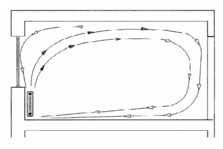
Example of convective movements caused by a radiator
