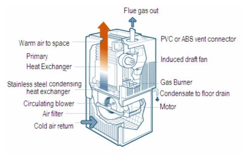
High Efficiency Condensing Gas Furnace
