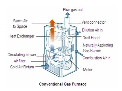
Note that there are two entirely separate air movement paths: first, the combustion path supplies air to the burner and to the draft hood and carries hot combustion gases through the burner, heat exchanger and flue pipe to the vent outdoors and second, the heat distribution and cold air return path circulates and heats the air indoors.
