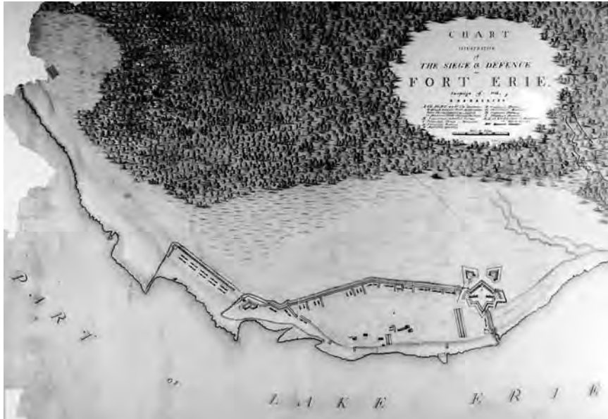
Map of Fort Erie depicting how Army engineers changed the old British fort into a bastioned work
